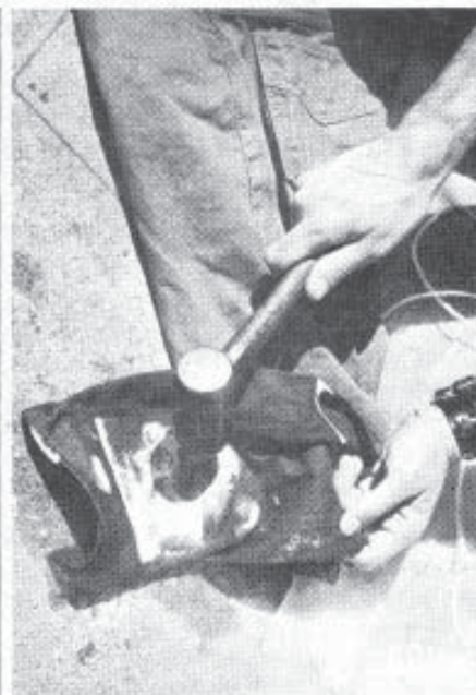
The frigid area was struck with a hammer during "Freeze Test."
